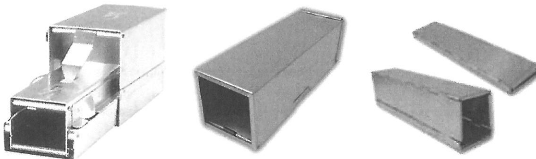
Figure A1. Examples of traps used, from left to right, Longworth trap, Sherman non-folding trap and Sherman folding trap.
