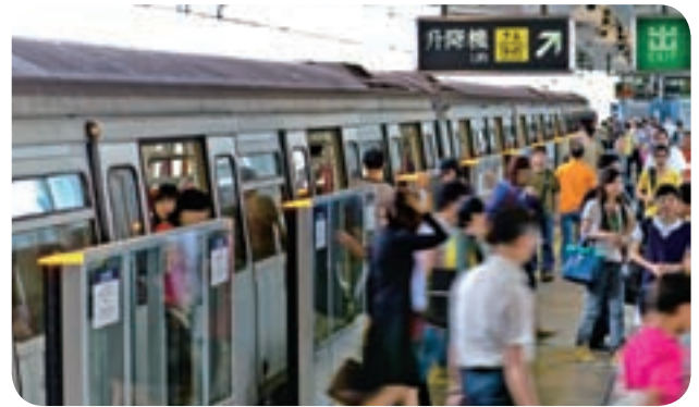
New automatic platform gates to improve platform conditions
