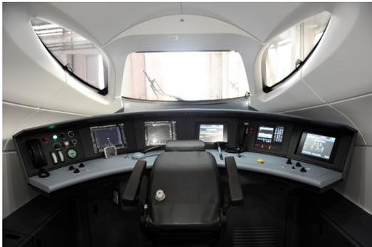
The driving cab located at both ends of the train include a driving console to control traction & braking systems, the train information system, train-borne signalling system and communication system, etc.
