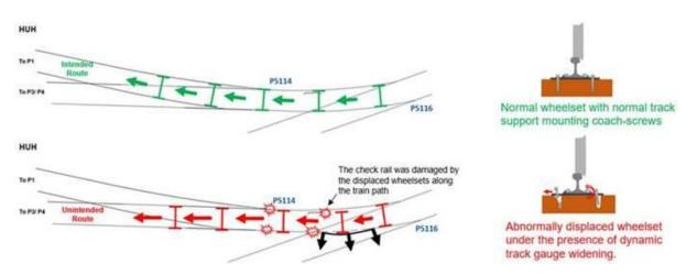
\* Check rail is laid parallel to a running rail to guide wheels through rail crossing of all turnouts
