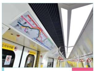
A tailored LED lighting system is being installed on our urban line trains, achieving up to 50 percentage energy savings relative to conventional lighting systems
