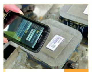
In our railway extension projects, a new smartphoneenabled materials-testing system is being used by workers at our five new lines construction sites
