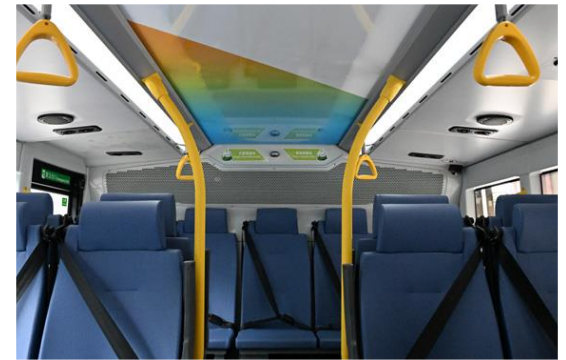
The roof of electric bus is equipped with solar panels to power the bus ventilation system and LED lighting is adopted
