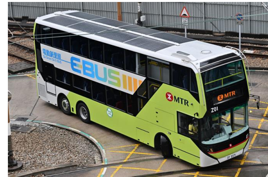
The roof of electric bus is equipped with solar panels to power the bus ventilation system and LED lighting is adopted
