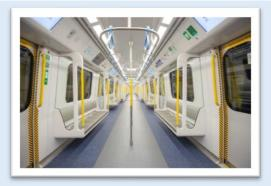
Train bodies are about 12cm wider than that of the existing trains, providing a more spacious travelling environment and narrowing the platform gap
