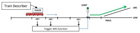
The TD would step forward as the physical train moves forward. As the train passes the signal, the signal aspect would be turned to Red and TD steps across the signal. The route set will be released as train passed the route.
