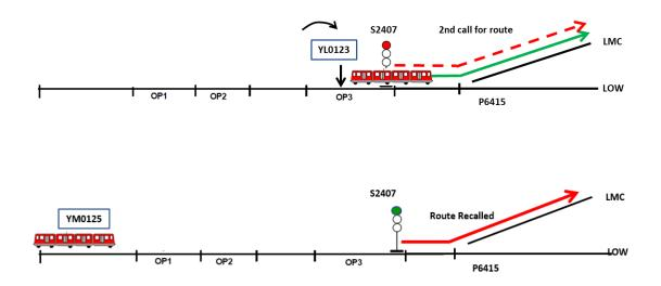
Another side effect is, subject to the extent of the delay "TD stepping", false SPAD alarm may be resulted in TMT processing when the delayed TD steps across a red signal:
