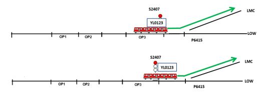
As the following train YM0125 approaches with Red signal aspect and no route ahead, automatic route setting for it will occur when its TD steps on OP1, leading to its own destination to LOW as defined by TD.
