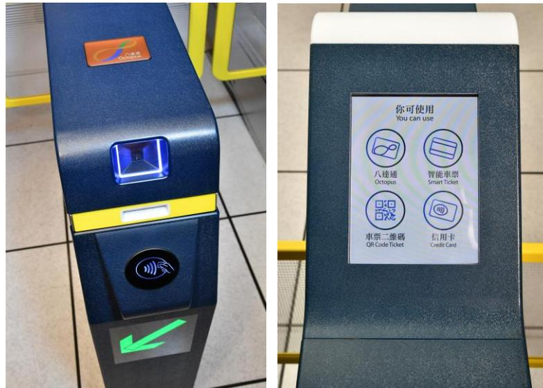
2. The new gates feature a flap design with a slimmer gate body than the existing tripod turnstile gates, making walkway for passengers wider. Besides smoother entry and exit for passengers, there will also be added convenience for those travelling with baby prams, trolleys and luggage.
