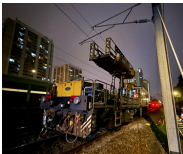
Figure 2: The Incident Overhead Line Inspection Vehicle
