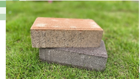
Trial on making eco-paver by upcycling spoil ballast generated from East Rail Line ballast replacement project.
