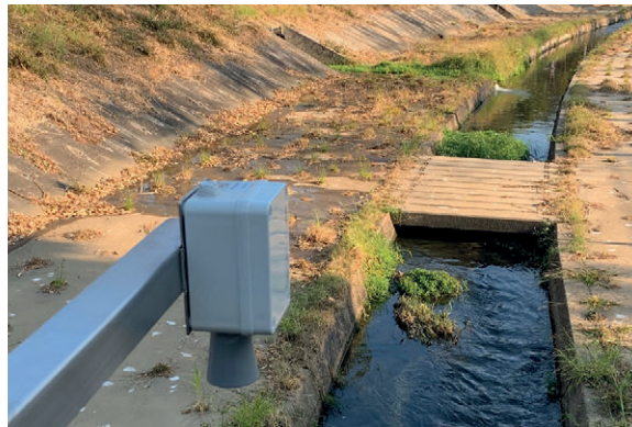
Water level sensor can provide real-time monitoring of the water level at rivers and channels
